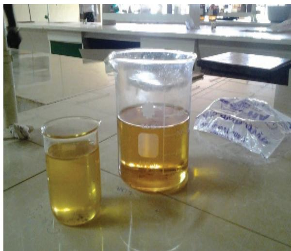
**Fig. 1a.** Low FFA oil after acid-catalyzed esterification
