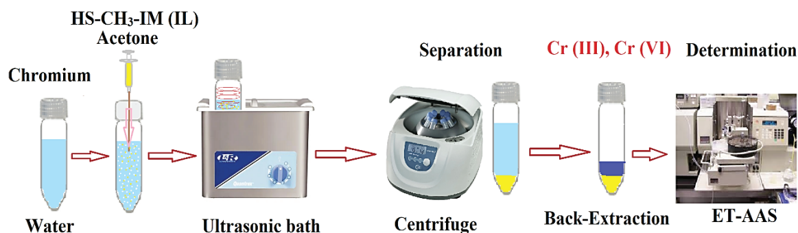
Fig.1. The extraction and speciation chromium based on \text{HS-CH}_3\text{-IM} by the USA —D-ILLME procedure
