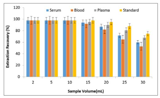
Fig.9. The influence of sample volume on lead extraction based on SM@NGO adsorbent by the SF-D-µ-SPE procedure
