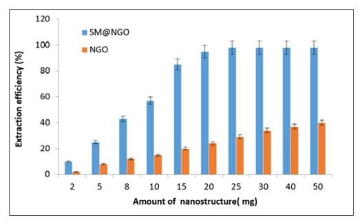
**Fig.8.** The influence of amount of SM@NGO on lead extraction by the SF-D-μ-SPE procedure
