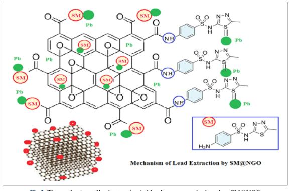
Fig.2. The mechanism of lead extraction in blood/serum samples based on SM@NGO by the SF-D-µ-SPE procedure
