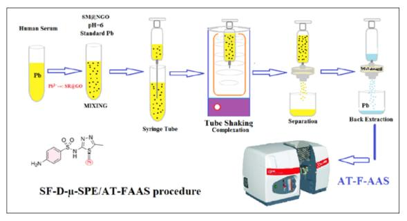
Fig. 1. The SF-D-µ-SPE procedure for extraction of lead in human samples
