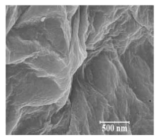
Fig.4. The SEM of SM@NGO adsorbent
