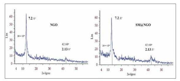
Fig.6. The X-ray diffraction (XRD) for NGO and SM@NGO adsorbents
