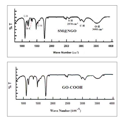
Fig.5. The FT-IR spectrum of NGO-COOH and SM@NGO adsorbent
