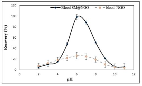
Fig.7. The influence of pH on lead extraction based on SM@NGO adsorbent by the SF-D-µ-SPE procedure
